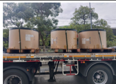
Fig. 2 : 3 coils were slide, displace from original position about 10cm. on pallet
